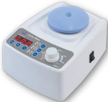
VM-01UA Vortex Mixer with Digital Timer and Analog Speed
