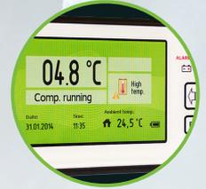
The user friendly G214 controller is standard for the ULUF 65. It includes different alarms as visual, acoustic, open door and more.
