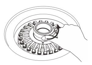
Place the wrench onto the knob and loosen the knob counterclockwise.
