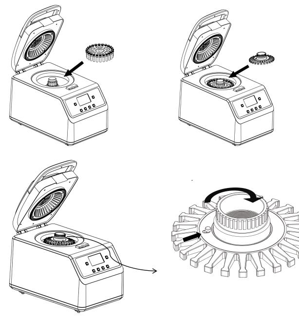
Tighten the knob clockwise, and pull the locking latch inwards to lock the tube retainer in place
