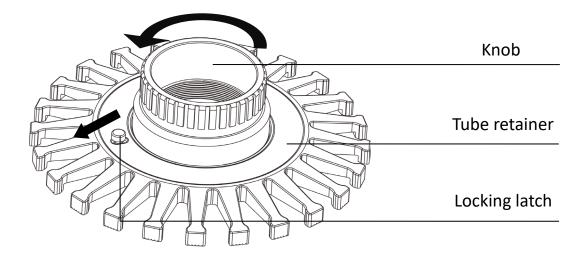
1.2 The tube holder maybe be filled in or out of the instrument. To remove, simply lift off the shaft. Place the tubes into the tube holder and press down until seated. If less than 24 tubes are used, they should be evenly distributed in the tube holder. If removed, the tube holder can then be replaced, making sure the two bumps on the holder line up with the indentations on the shaft.
