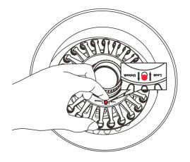
Move the lock lever outward to unlock the tube retainer. If the lock lever cannot be moved outwardly, please turn the knob for 2 degrees and turn the lock lever again.
