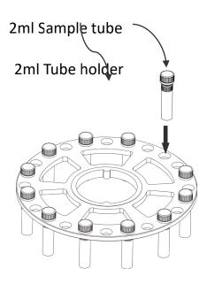
1.3 Place the tube retainer on top of the tube holder. Tighten the kiob clockwise and push the locking latch inwards. A click will indicate that the latch is in place. If the latch cannot be pushed inwards, turn the knob 2 degrees and try again.
