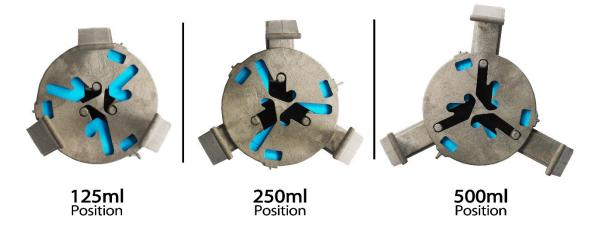
Once the clamp has been adjusted to the appropriate setting, place the clamp onto the **MAGic Clamp platform** in the desired platform location. The MAGic Clamp platform should consist of a steal base and a rubber mat. The platform is to be applied above the rubber mat.
