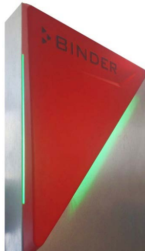
Figure 8: Display of the signal triangle (operation without any problems)
