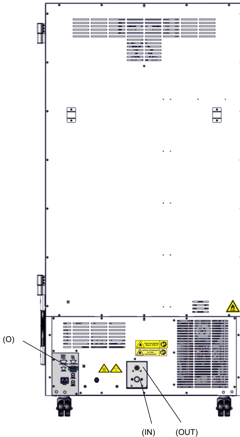
Figure 11: Rear view of the chamber with water connections
