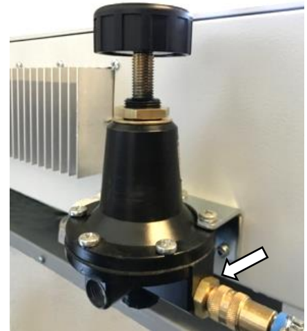
Figure 12: Compressed air connection on the pressure regulator
