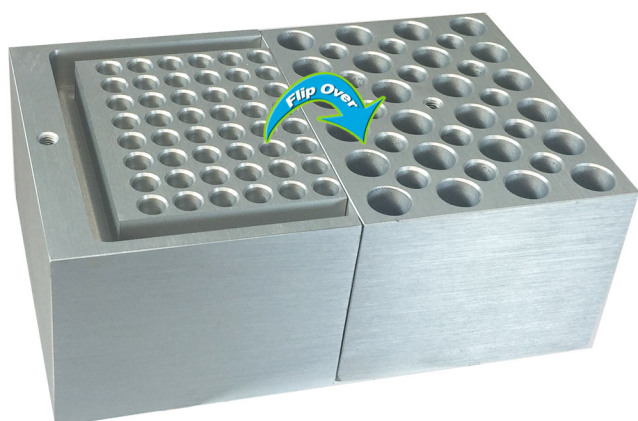
Catalog Number: BSWHEM Capacity: 48 x Hematocrit tubes Block Dimensions: 3.75 x 3 x 2 inches Hole Dimensions: 1.8 x 50 mm
