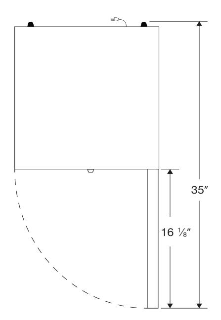
Note: This unit must have 4" clearance on sides and back for adequate ventilation
