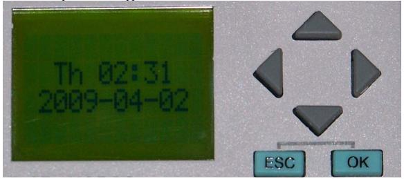
3. To change the preset cycle times, press "ESC". The option screen will appear.
