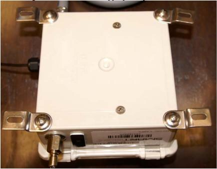
3. With the mounting brackets moved, position the unit in the appropriate location on the wall and mark the two holes. Remove unit from wall and drill the holes. Secure the unit to the wall with appropriate screws. (Wall screws are not included.)
