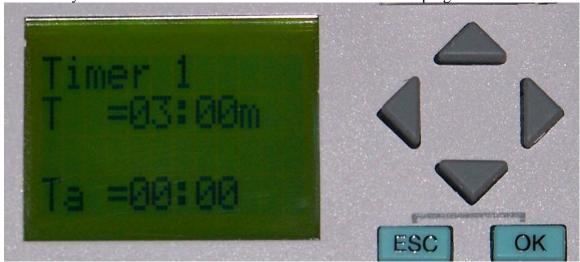
6. The EA-32002C offers two programmable timer settings. Press the up/down keys to navigate the timer choices. When the desired timer appears, repeat step five to change the time.
