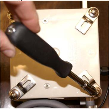
2. Using a Phillips head screwdriver loosen the screws and move the mount tabs outward as pictured below. Tighten the screws once appropriate position is achieved.
