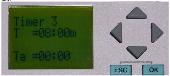
7. After setting the timers, press the "ESC" button twice to return to the opening screen. The Lab Control Unit is now ready to operate. Close and latch the door.
