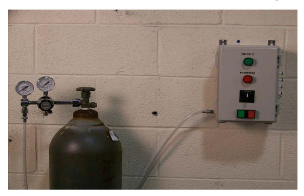
5. Connect the supplied cage hoses from the outputs of the Lab Control Unit to the input valve on the Euthanex Lid(s). To properly make the connection, pull back the coupler and slide it over the male stem. The coupler will snap back into place and secure the connection.
