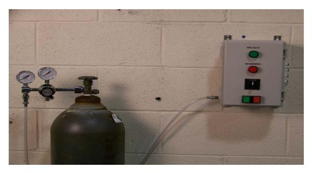
2. The EA-34000 offers four distinct timing choices. Select the desired timing cycle on the timing selector switch. Longer timing cycles are recommended for multiple cages or when treating larger animals.
