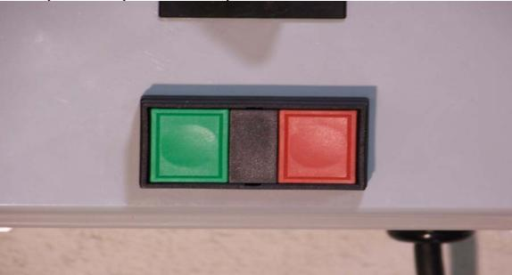
5. The cycle may be stopped at any time by pressing the red "Stop" button. This immediately stops the flow of gas.
