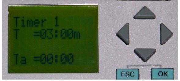
6. The EA-34000 offers four programmable timer settings. Press the Up/Down keys to navigate the timer choices. When the desired timer appears, repeat step five to change the time.
