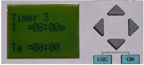
7. After settings the timers, press the "ESC" button twice to return to the opening screen. The Lab Control Unit is now ready to operate. Close and latch the door.
