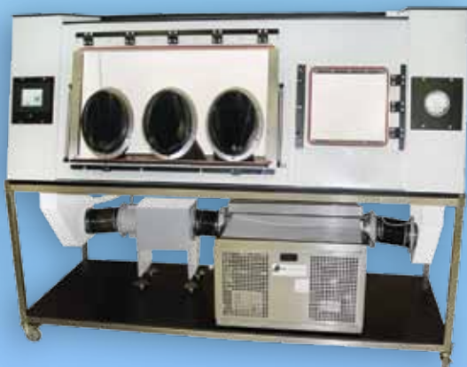
TEMPERATURE AND HUMIDITY CONTROLLED ENVIRONMENTS (THCE)
