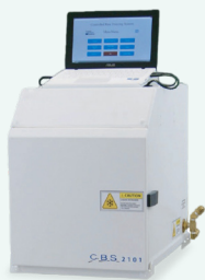
2101 Controlled Rate Freezer 28-Liter Capacity
