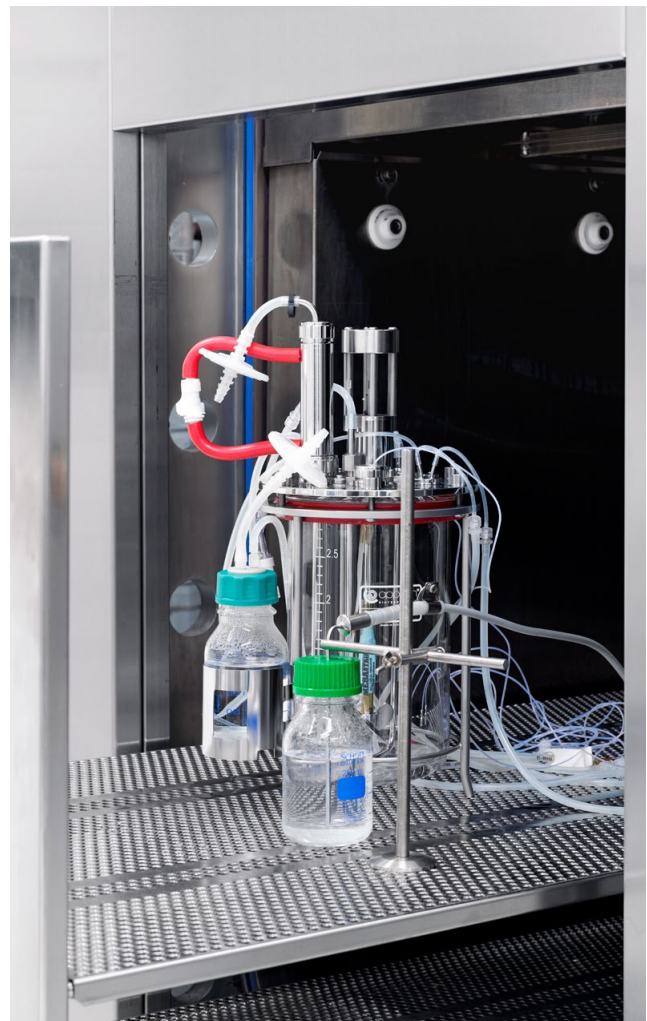
Once the bioreactor and associated components are cleaned, a programmable sterilizer cycle assures final preparation in compliance with protocols essential for validation.
