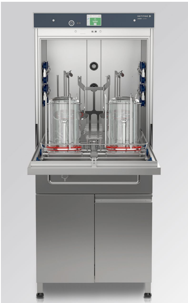
Getinge Lancer Ultima laboratory washer model 910LX loaded with 3L bioreactor in wash rack.
