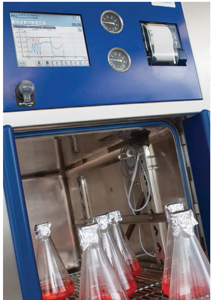
The AVANTI User Interface plot graph displays temperature and pressure performance over time.
