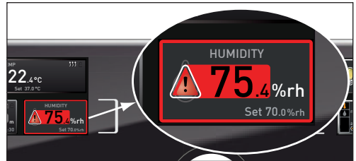
Fig. 21 Humidity monitoring triggered
