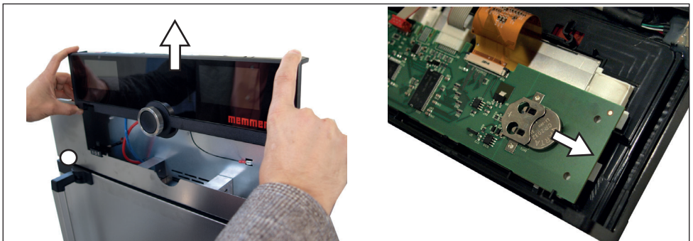
Fig. 34 Removing the lithium battery
