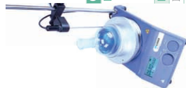
MS-H-Pro + with PT1000 and reaction block
