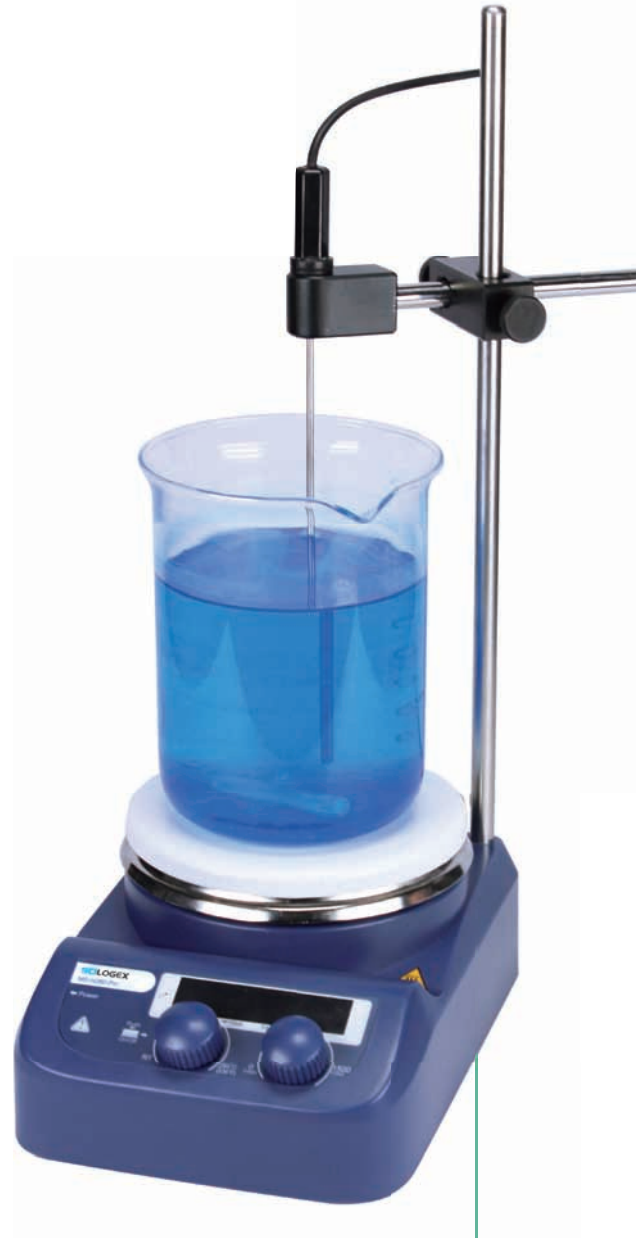
MS-H280-Pro BlueSpin with external temperature sensor PT1000
