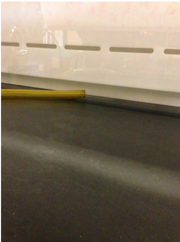
P.A.O. challenge introduced into cabinet workzone center rear wall
