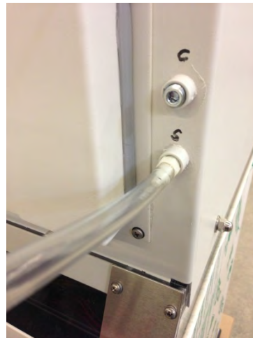
Gross leak sample taken from the primary HEPA filter
