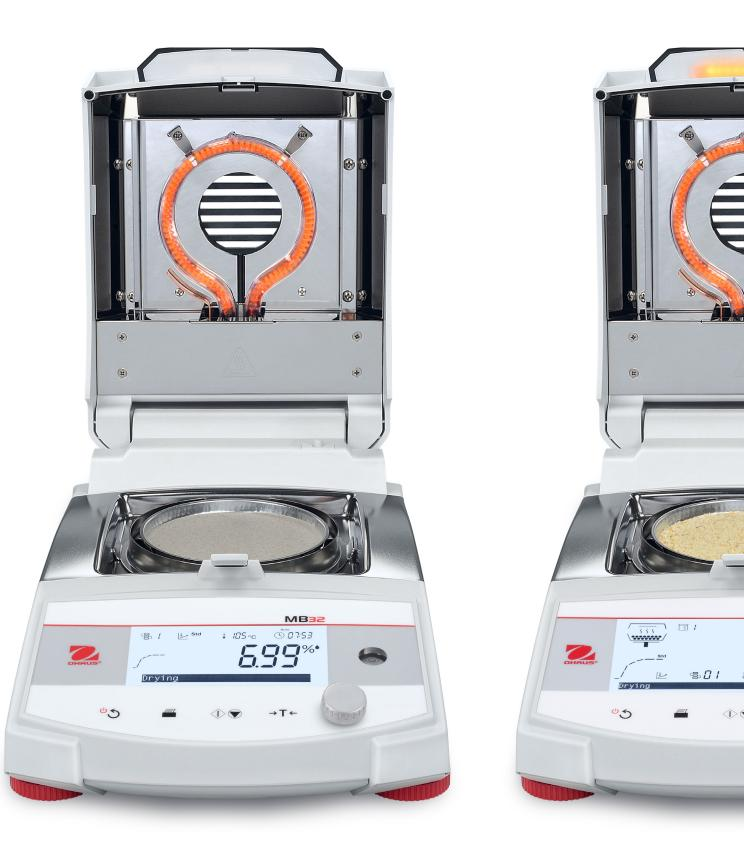
The MB32 is ideal for routine moisture testing, providing consistent performance for everyday laboratory and production needs. The MB62 is ve suitable for a v moisture appli different indus
