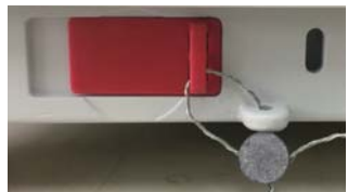
Locked with Wire Seal
