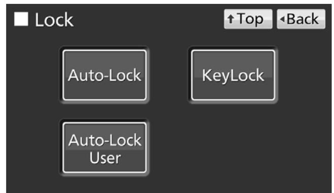
4. On the Auto-Lock User screen, it is possible to register a User-ID and its password. Press Apply key to save the User-ID and its password.
