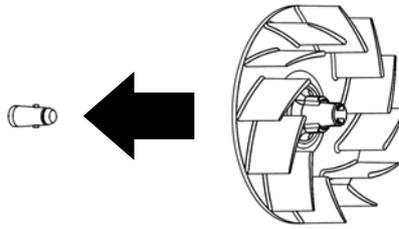
2. Lightly turn the fan manually to make sure that it does not touch the rear panel.
