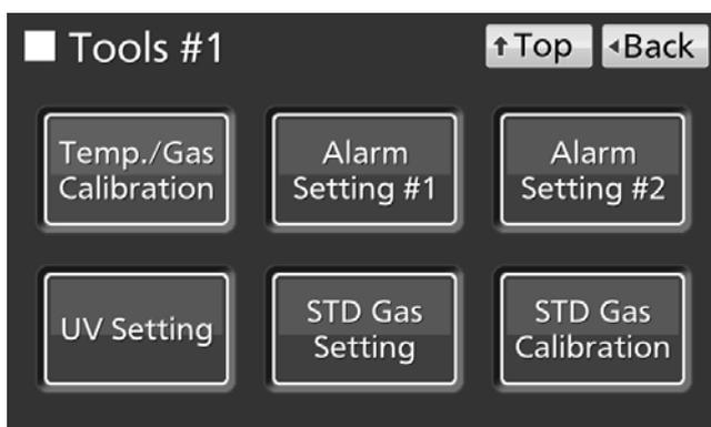
7. On the UV Setting screen, by holding the UV 24h Mode slide key and sliding it right, the UV 24h Mode is turned to ON. Press Apply key to start the UV 24-hour mode. The display returns to the Tools #1 screen.
