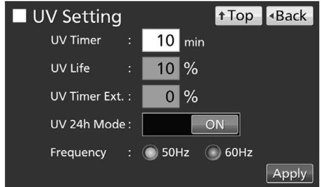
8. The UV lamp lights continuously for 24 hours. "UV : ON" is displayed on the UV lamp condition display when UV lamp is lighting.
