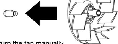
2. Lightly turn the fan manually to make sure that it does not touch the rear panel.
