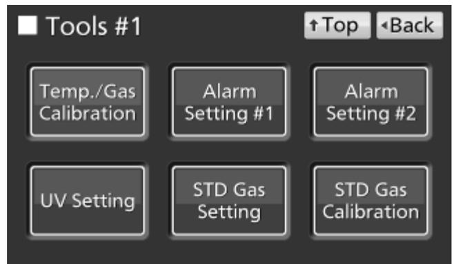
4. On the Alarm Setting #1 screen, input each parameter. Press Apply key to save the input value. The display returns to the Tools #1 screen.
