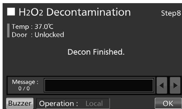
18. After  $\text{H}_2\text{O}_2$  decontamination, surplus  $\text{H}_2\text{O}_2$  liquid will remain at the bottom of the chamber and in the bottom part of the  $\text{H}_2\text{O}_2$  generator duct. This solution contains  $\text{H}_2\text{O}_2$  at a low density, so put on protective glasses and rubber gloves and wipe it up with a non-woven cloth.
