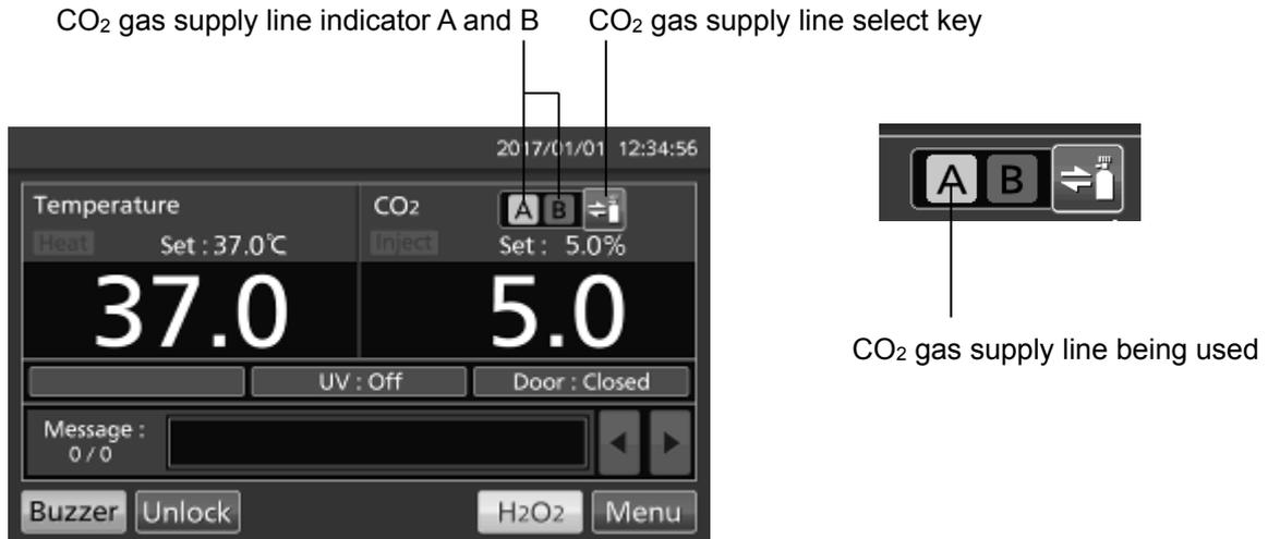
When the CO<sub>2</sub> density level remains unchanged, even though the CO<sub>2</sub> gas valve in the unit is opened, the unit regards the present connecting CO<sub>2</sub> gas cylinder as an empty. The CO<sub>2</sub> gas supply line is changed over automatically. These movements are displayed (Table. 2).
