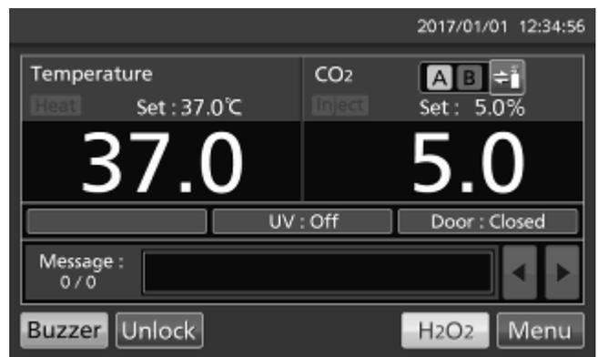
2. Press Lock key to lead the Lock screen.
