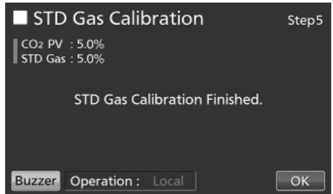
11. On the STD Gas Calibration Step5 screen, press OK key to return to the Tools #1 screen. On the Tools #1 screen, press Top key to return to the Top screen.
