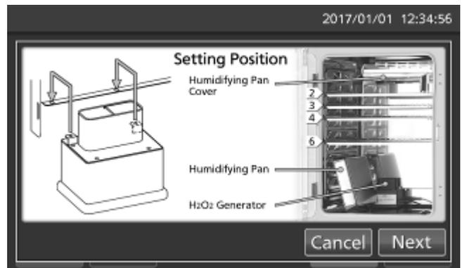
13. On the H<sub>2</sub>O<sub>2</sub> Decontamination Step1 screen, the system check starts automatically. If the system is normal, the display leads the H<sub>2</sub>O<sub>2</sub> Decontamination Step2 screen. When the system is abnormal, refer to Table 8 on page 85.
