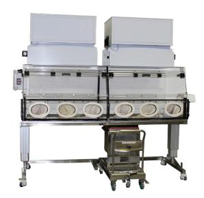
Sieving Suite Hybrid Isolator designed to house Retsch AS–200 TAP Sieve Shaker and Hirschmann Laborger te Jolting Volumeter STAV–II with Water bath cart. Airfoils and plenums coupled with a BIBO (Bag–In/Bag–Out) dual HEPA filtration system control airflow across the workstation and maximize personnel protection while working with powder APIs. Stainless steel construction with inset acrylic paneling allows for ambient light transmission. Size
