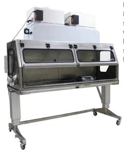
Bulk Powder enclosure with side—mount EHS—Now Drum Lift System. The unit features a top—mounted HEPA filtration system and is designed for personnel protection while working with powder substances. Unit designed to contain balance application. The enclosure features an acrylic superstructure and side panels with a hinged door. Also features a waste chute.
